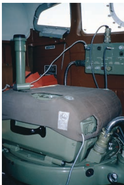
Photo 5 Aerial camera, RC-9, installed in a Cessna
