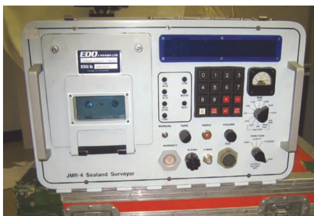
Photo 6 NNSS observation equipment (JMR-4A)
