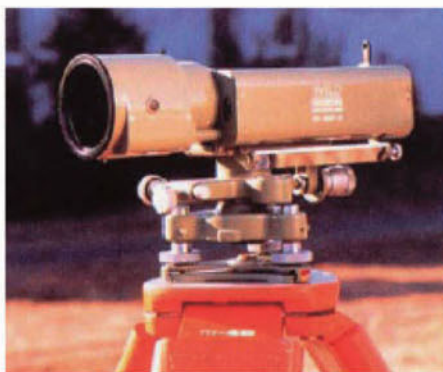
First-class level N3 (tilting level)
